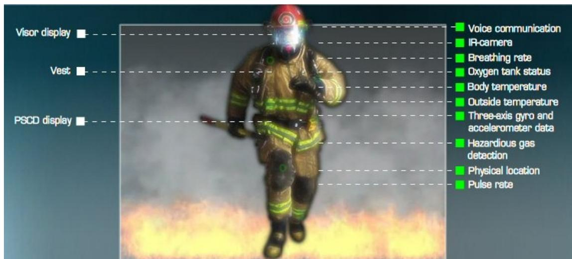
Figure 2: The fire fighters of the future will be equipped with interconnected devices to provide more data about the hazards they face and to monitor their own safety during rescue work
